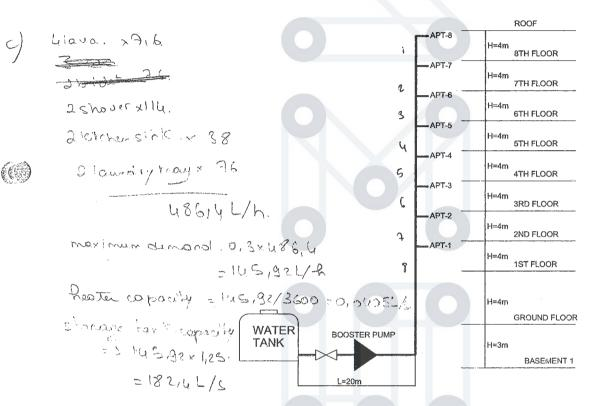
Each floor level is 4m height; the ground floor is a reception area, the water tank and the booster set are located in basement floor. (For pipes lengths and floors heights refer to schematic riser)
